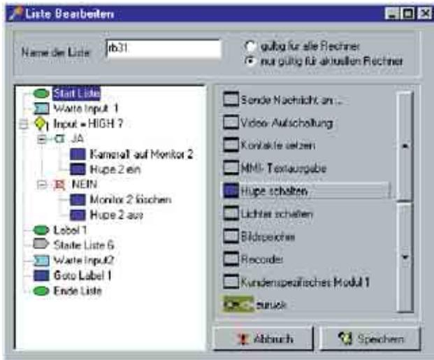
The Event Manager is a simple, effective tool for creating project-specific automated functions. The Event Manager's menus behave just like those of a standard object and it produces customised functions quickly and easily by setting parameters rather than by programming.
