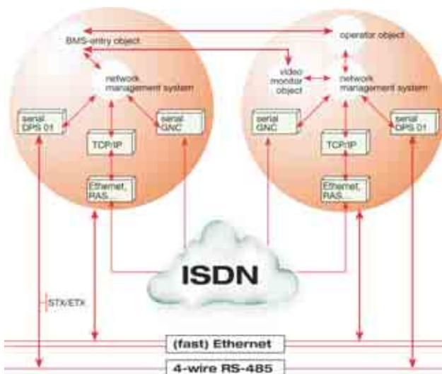
In pletta open security architecture a specially developed communications and network management system takes over management of communication between objects. It provides open communication with the ability to use many different transmission media. New transmission systems can be included by simply replacing the driver.
