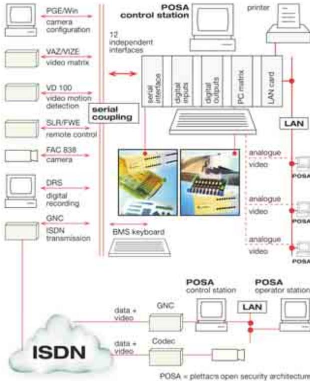
The technology of plettac open security architecture (POSA) supports many different types of link between modular, autonomous control units, so that a complex network of transmission paths and a highly efficient, customised solution can be created.
