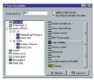
The Event Manager is a simple, effective tool for creating project-specific automated functions. The Event Manager's menus behave just like those of a standard object and it produces customised functions quickly and easily by setting parameters rather than by programming.
